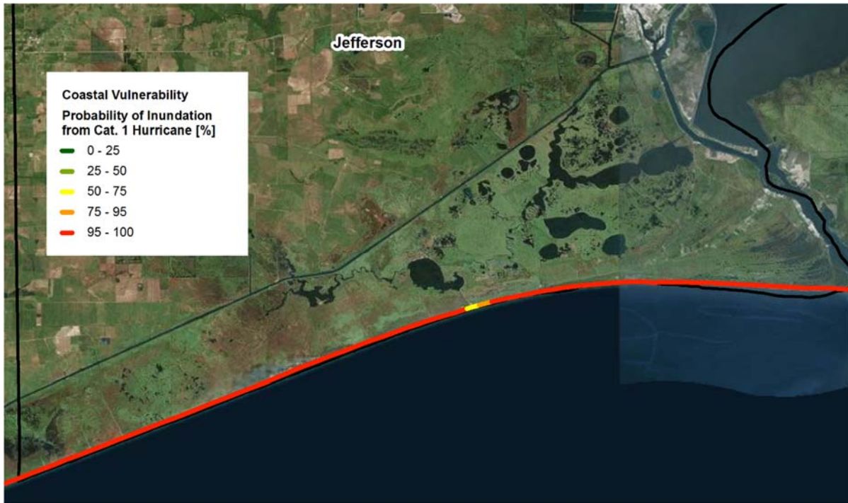
Figure 27: Probability of coastal inundation from category 1 hurricane landfall (Doran et al., 2016)
