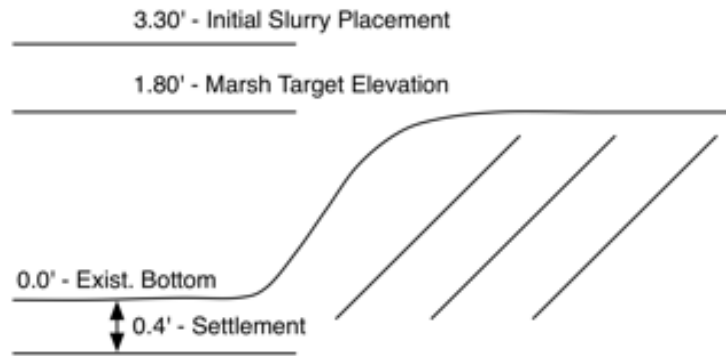
Figure 38: Cartoon showing key elevations used for the computation of marsh nourishment quantities
